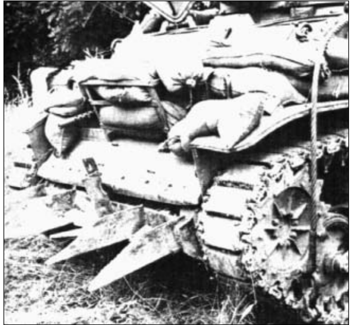
Technical innovations helped turn the tide in Normandy. A Sherman tank is equipped with a hedgerow cutter constructed of materials from German beach obstacles. Invented by Sgt. Curtis G. Culin of the 2nd Armored Division, the “rhino” device was a huge benefit to our tanks in hedgerow combat.
